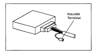
4. Secure the wire and terminal to the outside of the wire harness using vinyl electrical tape.
