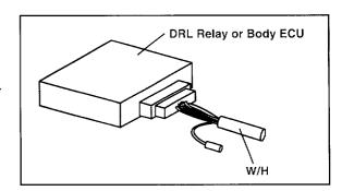
3. Insulate the removed terminal using vinyl electrical tape.
